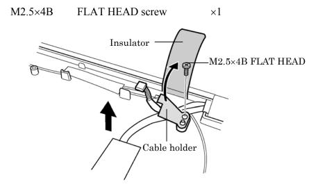
Figure 4-44 Removing the cable holder
